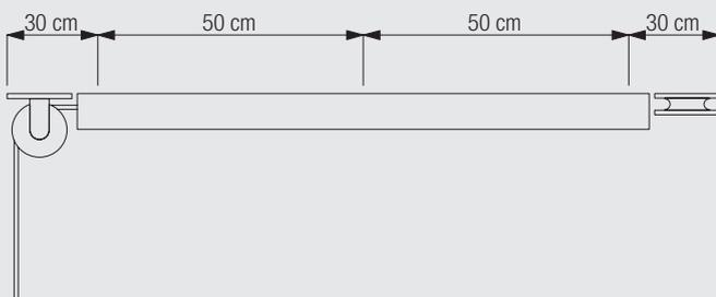
This motor is enormously strong and both fixing points and ceiling must be accordingly solid. Timber soffit at least 4cm thick over complete length of track is recommended.
