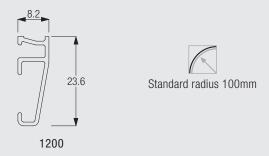
The standard radius is recommended for optimal operation.
