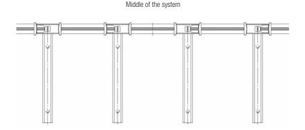
Align the shells according to the position of the loop tapes. The arrows on the shells must be in line with the loop tape / rings.
