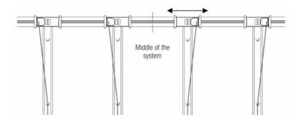
Once the system has been installed check that the cord is winding neatly onto the spools.
