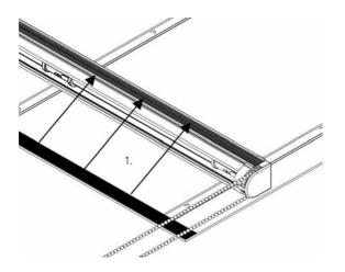
Lay the fabric on his front side and lay the system on the fabric like shown.
