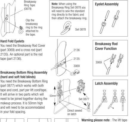
Warning please note : The lift tape of cord should be taut against the rear of the fabric when the blind is in the fully lowered position. The tapes and cord should always be central within the 0877 breakaway device.
