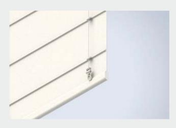
The new legislation also affects the inner cords of Roman blinds. If the attachment/retention points (lift points), are over 200mm apart they must have some form of breakaway device.
