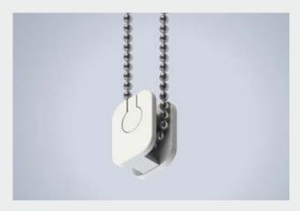
The cord retainer is a fixed tensioning device which ensures operating cords and chains are kept taut therefore not creating a hazardous loop. They need to be fixed to a surface (normally a wall) at the maximum distance possible from the headrail.
