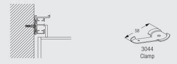
Clamp 3044 requires additional fixing with a small screw for maximum security.
