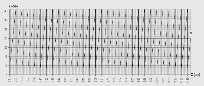
Due to technical reasons there will be a light gap (y) on the front side of the system. The size of the gap depends on the length of the system (x). If required, this gap can be hidden with a special faceplate (fitting on site).
