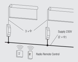
Details of radio control parts and accessories can be found within the Switches section of the catalogue.
