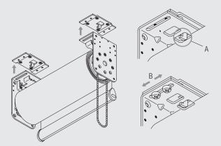
Specially designed pre-fitted hook-in plates 4972 (A) take the weight of the blind whilst the fitters carry out final detailed positioning (B) of the brackets. The brackets can be sideways adjusted by up to 18mm. This unique feature is very well received by all fitters around the world.
