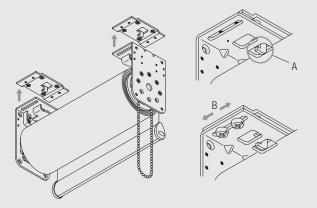
The brackets can be laterally adjusted by up to 18mm.
