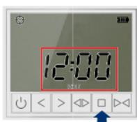
3. Press stop function to enter timing setting window
