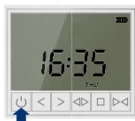
6. Press function button and hold for 3s, then back to control window
