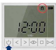
1. Press function button for 3s to enter control window
