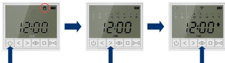
1. Press function button for 3s to enter control window
