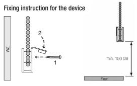
This retaining device should be installed at the maximum distance possible from the control mechanism to prevent the looped pull cord(s) becoming slack.
