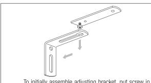
To initially assemble adjusting bracket, put screw in end topplate position on 'arm'. Locate screw head through key hole on fixed (base) bracket.
