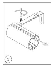
Offer track up to wall and mark a point 7cm (2³/4") std except 5.5cm on 6120/6160 from each end using the 3rd position on the end set support. Firmly fix brackets to wall in these positions. Fix remaining brackets to wall at equal intervals between these brackets (approx. 60cm/2'0") ensuring that they are perfectly level.
