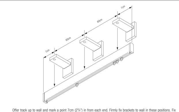
remaining brackets to wall at equal intervals between these brackets (approx. 60cm/2'0" apart) ensuring that they are perfectly level.
