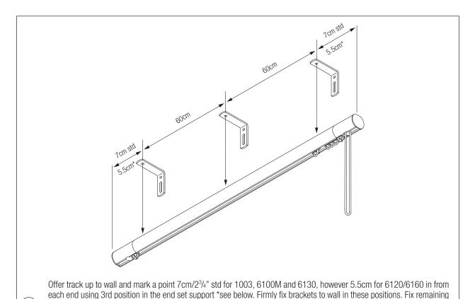
brackets to wall at equal intervals between these brackets (approx. 60cm/2'0") ensuring that they are perfectly level.
