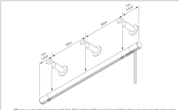
Offer track up to wall and mark a point 7cm ( $2^3$ / $4^n$ ) std for 6130 except 5.5cm 6120 in from each end using the 3rd position of the end set support. Firmly fix brackets to wall in these positions. Fix remaining brackets to wall at equal intervals between these brackets (approx. 60cm/ $2^n$ 0 a part) ensuring that they are perfectly level.
