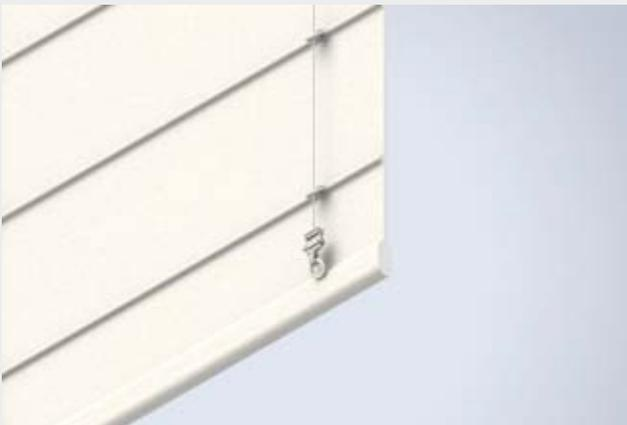
The new legislation also affects the inner cords of Roman blinds. If the attachment/retention points (lift points), are over 200mm apart they must have some form of breakaway device.
