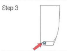
Remove magnet when LED starts to flash Module is now in set-up mode
