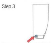
Remove magnet when LED starts to flash Module is now in set-up mode
