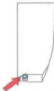
Remove magnet when LED starts to flash
