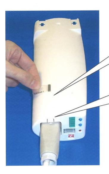
Magnet position is in line with the plug locating clamp and approximately 5 cm from the base of the motor.
