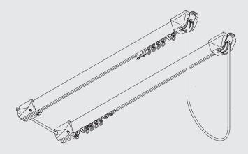
Used as parallel system with one cord pull only and infinite overlap it is ideal for stages. Refer to Fitting Options for fixing instructions.
