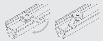
Allow about 20mm clearance from the wall for clamp rotation.
