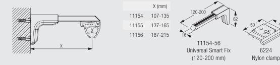
Brackets feature thread for screw M4x12 for fixing bracket SG 6224.
