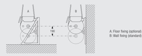
The steel core rope is tensioned by using the motor weight. Vertical variation possible up to 190mm. Minimum distance from track to motor is 2m.
