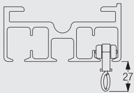
Diagram uses standard glider measured to the inside of the glider eye.
