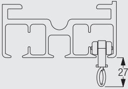
Diagram uses standard gliders measured to the inside of the glider eye.
