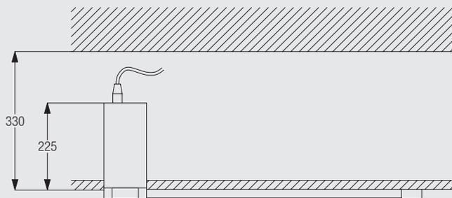
With profile surface mounted on the ceiling.
