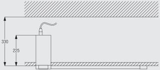
With profile surface mounted on the ceiling.
