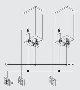
A: 230V/115V mains individual supply and switch All cabling between switch and motors is to be 3 core + earth B: Low voltage simultaneous (24VDC 3 core) C: Low voltage individual (24VDC 3 core)
