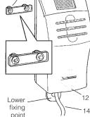
Drill holes (6mm masonry drill), insert wall plugs provided, screw fixing plate (16) to wall.
