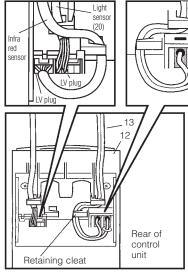
The control unit (12) is fixed to the wall by means of the fixing plate (16) and lower fixing point.
