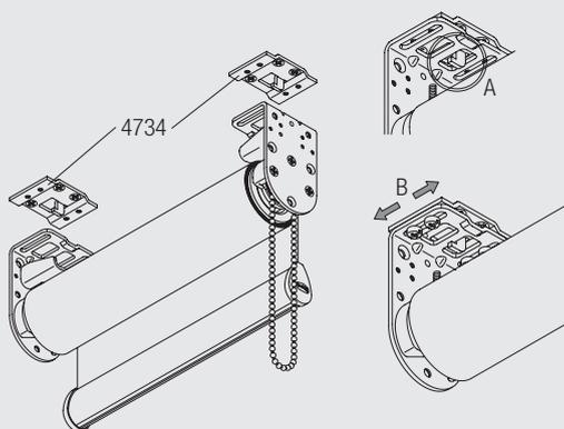
The brackets can be laterally adjusted by up to 15mm.
