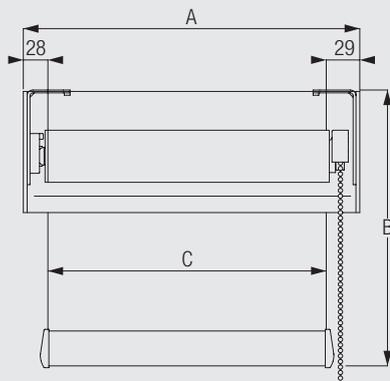
A: system width (= standard width + 8mm)
