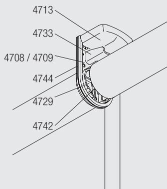
4708 Connection bracket for wall fixing
