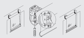
Vertical adjustment of the system (A) allows the head tube to be levelled.
