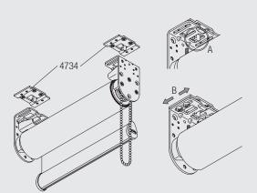
The brackets can be laterally adjusted by up to 15mm.
