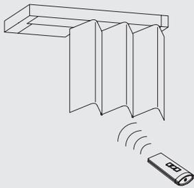
System with Silent Gliss motor 9091 features an integrated receiver and can be combined with Radio Remote Control Systems Silent Gliss 9940/0450 with minimum wiring. For further details, please refer to catalogue section "Motors & Controls".
